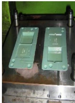
*Illustration 2. Metallic cavity and mold printed in 3D*
