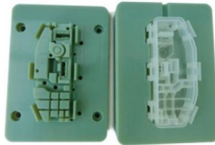
*Illustration 1. Plastic injection mold built by additive manufacturing and injected part*
