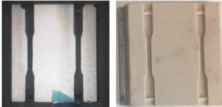
*Illustration 4. Test pieces and mold after 100 injections*
