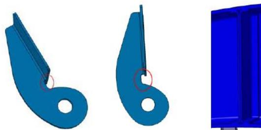
*Illustration 3. Examples of aircraft parts, currently in metal, that could be manufactured in ADDSET by thermoplastic injection*
